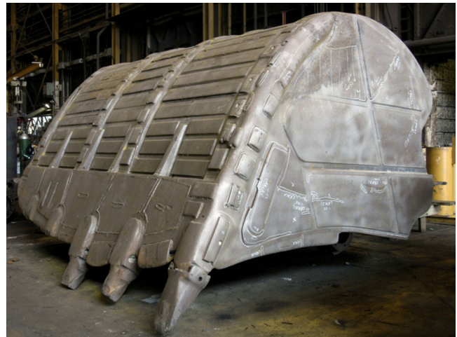
Figure 1. Large Mining Bucket Needing Repair
